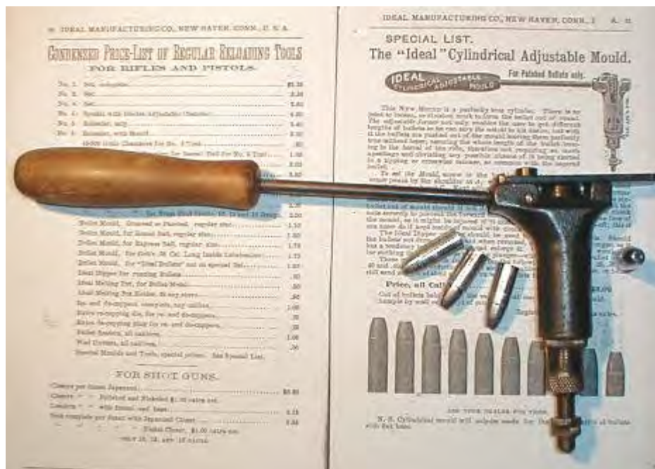
Figure 11: Ideal Cylindrical / Adjustable One-Piece Mould
