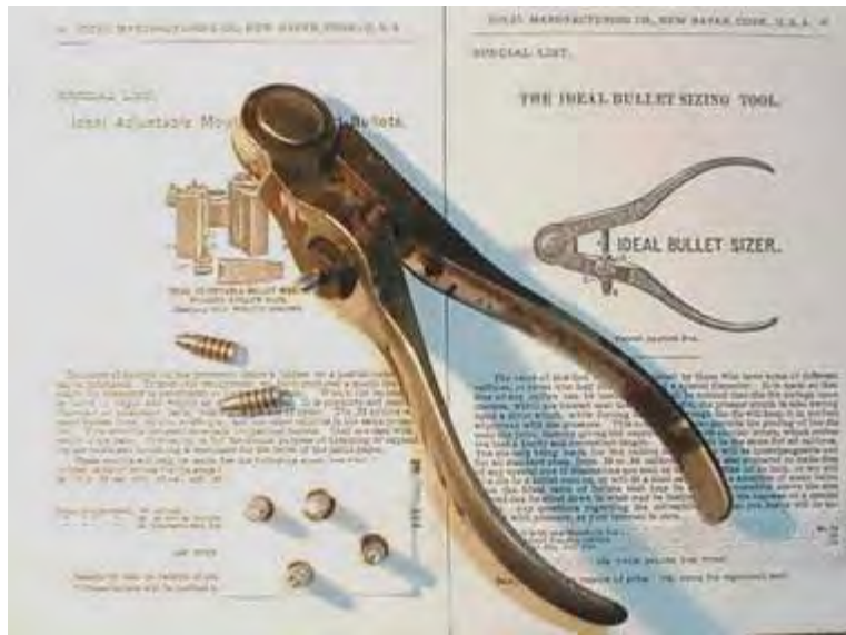
Figure 8: Ideal Interchangeable-Die Bullet Sizer
