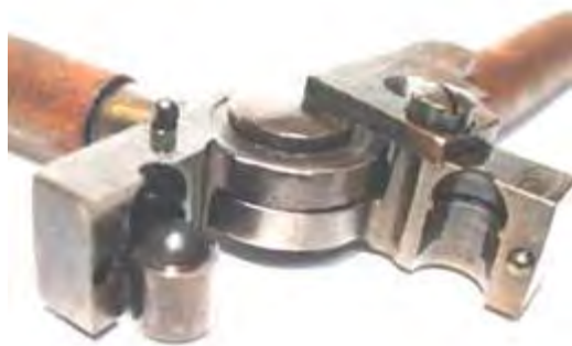
Figure 23. #429104 Hollow Base mould with fixed HB pin. This was the earlier method of making HB moulds.
