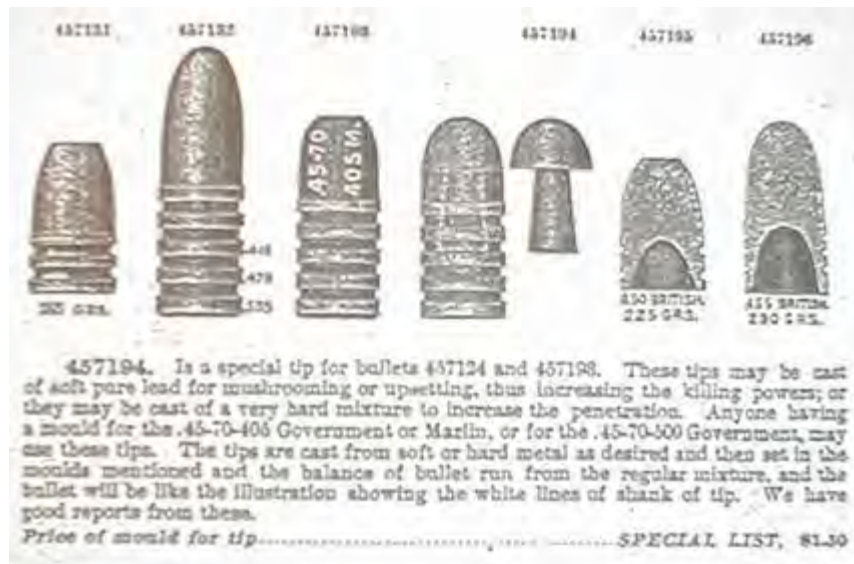
Figure 15: Ideal Soft- (or Hard-) Tip Mould for Government and Marlin .45-70 Bullets
