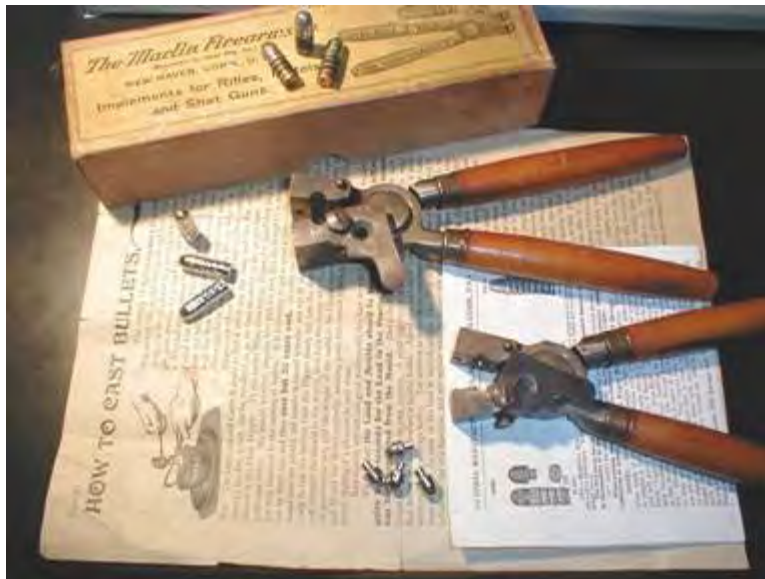
Figure 20. Marlin-made Ideal Body and Tip Mould Set for .30 Caliber Bullet No. 308291
