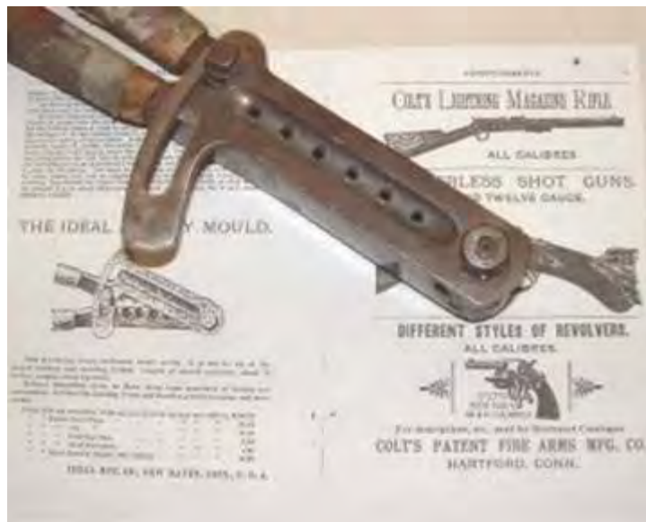
Figure 13. Early Ideal "Armory" Six-Cavity Mould
