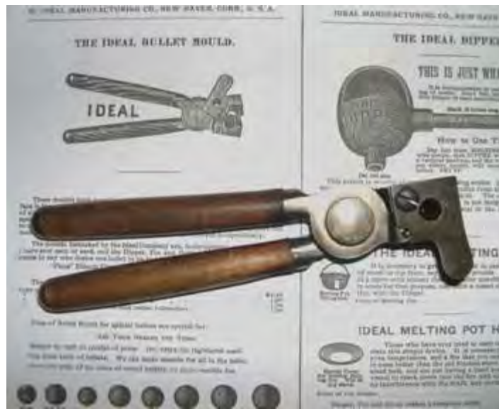
Figure 6: Early Ideal Mould with End-Capped Handles, no Ferrules Courtesy Marc Davison
