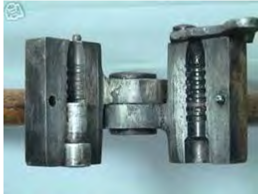
Figure 22. Perfection Mould modified for use as a "fixed weight" mould
