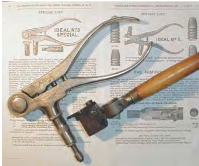
Figure 2: Ideal No. 3 Tong Tool with Double-Adjustable Seat/Crimp Die and Separate Ideal Mould
