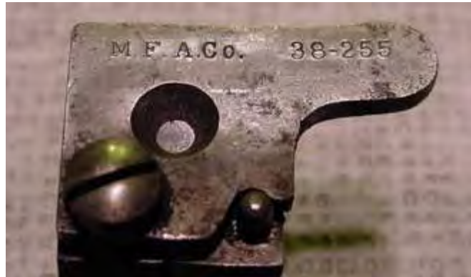
Figure 4: Early Ideal Mould with Ideal Address; Cartridge Designation Stamp
