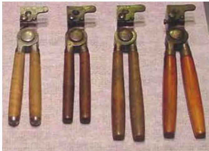
Figure 3: Early Ideal Moulds; Various Handle Patterns
