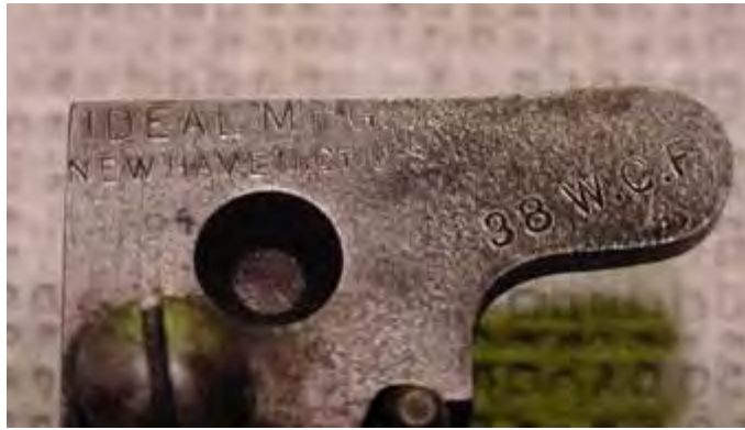
Figure 4: Early Ideal Mould with Ideal Address; Cartridge Designation Stamp
