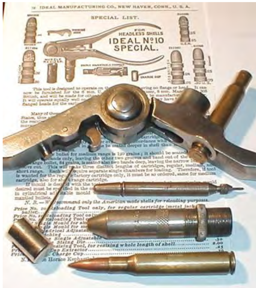
Figure 17. Ideal "No. 10 Special" Tool, .30-'06 Caliber for Spitzer Bullet
