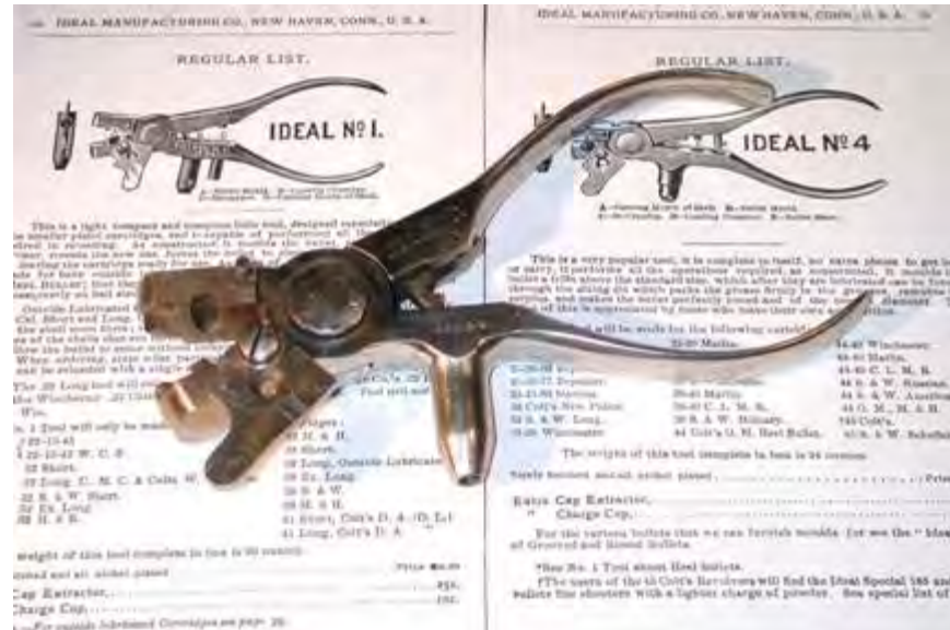
Figure 1 Early Non-Adjustable Ideal No. 1 Tong Tool with Integral Mould (Courtesy Tom Quigley)
