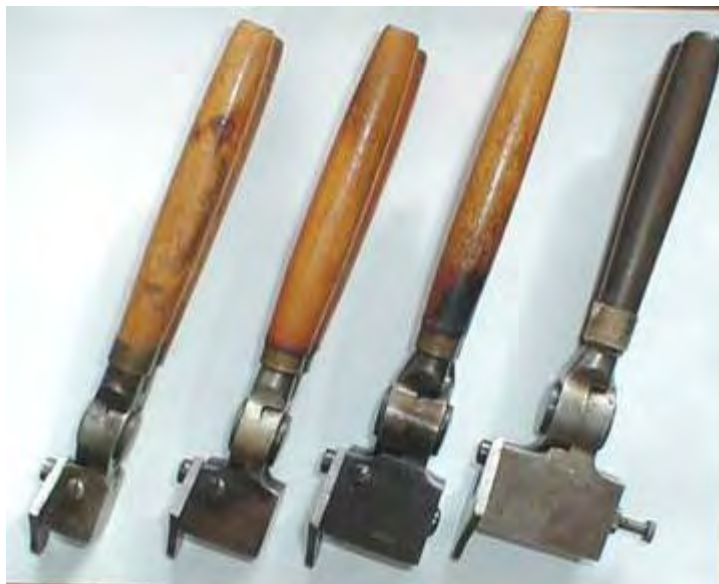
Figure 14. Standard Ideal Moulds, Various Block Depths
