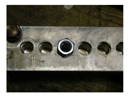
Fill the cavity with WW alloy including the Nut and water drop.
