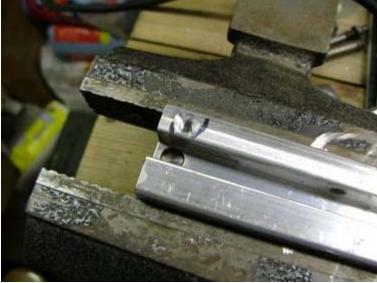
4.) Tap the hole using the 8-32 Bottoming Tap (since the hole is not open at the bottom. Again use small amounts of light oil and tap in stages emptying metal out of the tap as needed.
