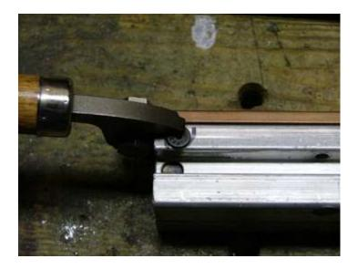
Fixing Handle Pins that fall out of the 2 Cavity molds
