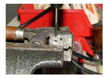
After tapping, Select a 6-32 screw to fill the hole, reattach the plate and use the set screw to hold the main screw to the appropriate tension.
