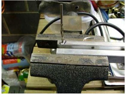
3.) Use the countersink in a drill to open the surface of the metal to hold the screw.
