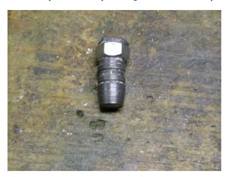
Coat the bullet with the provided clover compound and use a  $\frac{1}{2}$  inch box end wrench to twist the bullet in the cavities. You will need to recoat the bullet between cavities for best effect.
