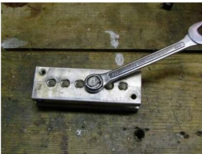
Clean the mold in Hot water then with Degreaser and re-assemble.
