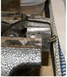
2.) Using the small of the two drill bit provided, drill a hole through the mold body into the sprue plate screw hole.
