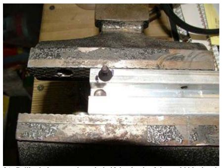
2.) Drill a hole approximately half the depth of the mold block using the larger of the 2 bits provided.
